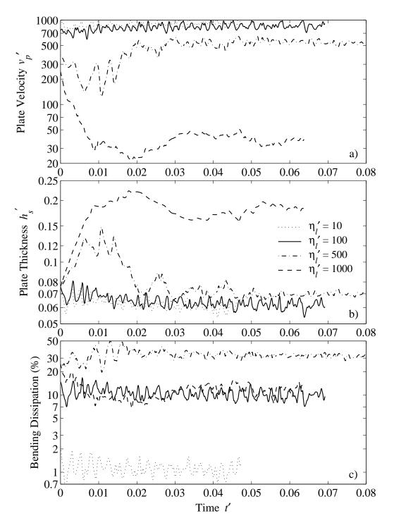
Figure 6.3: A comparison of (a) plate velocity  $v'_p$ , (b) plate thickness  $h'_s$ , and (c) the fraction of the total energy dissipation that occurs as plate bending within the subduction zone, as a function of time. Results are shown on a log scale for four subducting slabs with  $\eta'_l$  of 10, 100, 500, and 1000, for which  $Ra_m$  is  $1.1 \times 10^6$ ,  $1.2 \times 10^6$ ,  $1.5 \times 10^6$ , and  $2.9 \times 10^6$ .
