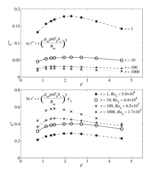
Figure 2.14: Plots of the dimensionless super-exponential growth rate, C'' or C', versus dimensionless wavenumber,  $k' = 2\pi/\lambda'$ , with time scaled using (2.11) in (a) and (2.29) in (b). Thus, (b) scales rates with "available buoyancy." We used an initially error-function temperature profile perturbed using (2.40) with p = 0.2.
