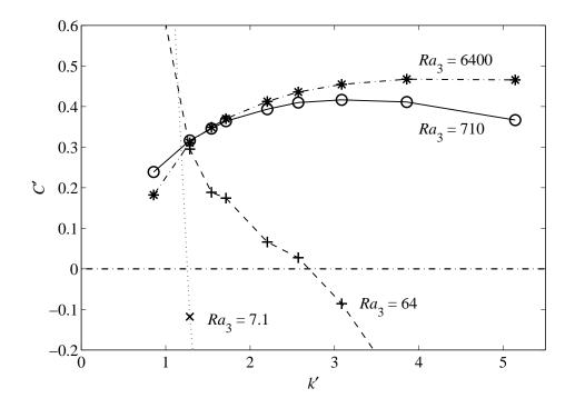
Figure 2.17: Plot of C' versus dimensionless wavenumber,  $k' = 2\pi/\lambda'$  for an initially linear temperature profile, perturbed using (2.40) and p = 0.2. All curves use r = 100, and  $Ra_3$  is varied by varying  $B_m$ . Time is scaled using (2.29) to include the "available buoyancy."
