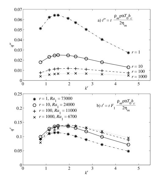
Figure 2.6: Plots of dimensionless growth rate, q'' or q', versus dimensionless wavenumber,  $k' = 2\pi/\lambda'$ , with time and length scaled using (2.11) in (a) and (2.29) in (b). Thus, (b) scales rates with the "available buoyancy." We used an error-function initial temperature profile perturbed using (2.40) with p = 0.04.
