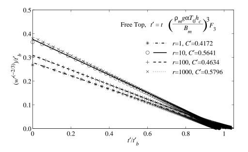
Figure 2.13: Similar to Figure 2.12b, but for free slip boundary conditions on the top surface, again using the "available buoyancy" to scale time. A comparison to Figure 2.6b shows that the "available buoyancy" scaling better accounts for the temperature dependence of viscosity if the upper boundary condition is free, rather than rigid.
