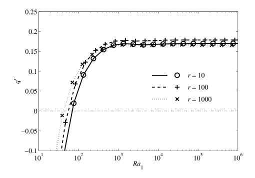
Figure 2.9: Plot showing how the dimensionless growth rate, q', varies with the stability parameter,  $Ra_1$ , for a layer with Newtonian viscosity (n = 1) and for r of 10, 100, and 1000. Scaling is with the "available buoyancy," as given by (2.29). A linear temperature profile, perturbed using (2.40),  $\lambda' = \lambda/h_l = 4.07$ , and p = 0.04 giving  $Z'_0 = 1.98\%$ , was used in each case, and we varied  $Ra_1$  by varying  $\eta_m$ .
