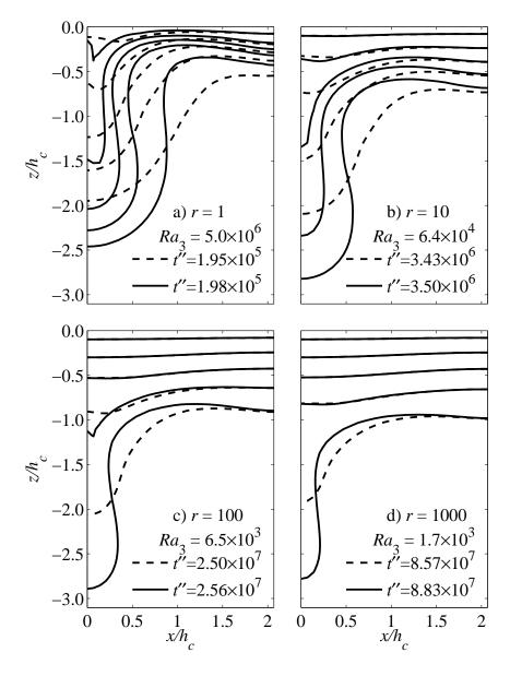
Figure 2.11: Similar to Figure 2.4, but for temperature profiles showing the growth of a convective instability in a non-Newtonian fluid (n = 3) from an initially error-function temperature profile that is perturbed using (2.40) with p = 0.2 and  $\lambda' = \lambda/h_c = 4.14$ . The times for both stages of the instability are given, and are scaled using (2.11), without the "available buoyancy."
