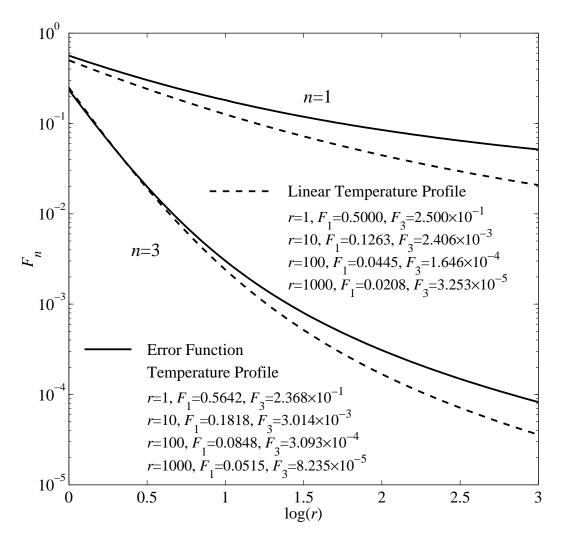
Figure 2.3: The total available buoyancy,  $F_n$ , as a function of  $\log r$  for both the errorfunction and linear temperature profiles, and for n = 1 and n = 3.  $F_n$  is calculated by integrating  $f_{ab}$  (Figure 2.2) according to (2.22). As the temperature dependence of viscosity increases with increasing r, more of the negative buoyancy becomes unavailable for driving a convective instability because of its increased strength. This is shown by the decrease of  $F_n$  with r.
