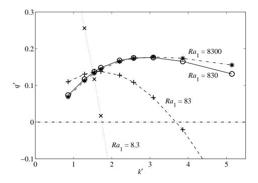
Figure 2.10: Plots of dimensionless growth rate, q', versus dimensionless wavenumber,  $k' = 2\pi/\lambda'$ , for an initially linear temperature profile, perturbed using (2.40) and p = 0.04. All curves use r = 100, and  $Ra_1$  is varied by varying  $\eta_m$ . Time is scaled using (2.29) to include the "available buoyancy."
