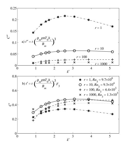
Figure 2.15: Similar to Figure 2.14, but for an initially linear temperature profile, perturbed using (2.40) with p = 0.2. Again, (b) scales time with the "available buoyancy," while (a) does not.
