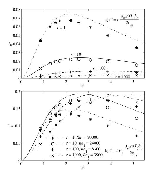
Figure 2.8: Similar to Figure 2.6, for an initially linear temperature profile, perturbed using (2.40) with p = 0.04. In this case, however, symbols show growth rates estimated from the finite element calculations and lines show growth rates predicted by Rayleigh-Taylor linear theory, as given by *Conrad and Molnar* [1997].
