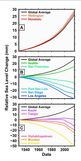
**Figure 2.** Model prediction of the relative sea level change caused by groundwater depletion since 1930. Here global average rise (black curves) is compared with trends at individual tide gauges (colored curves, labeled in order, locations in Figure 1) that are (a) far from depletion zones or close to regions of intense groundwater depletion in (b) western North America and (c) southern Asia.
