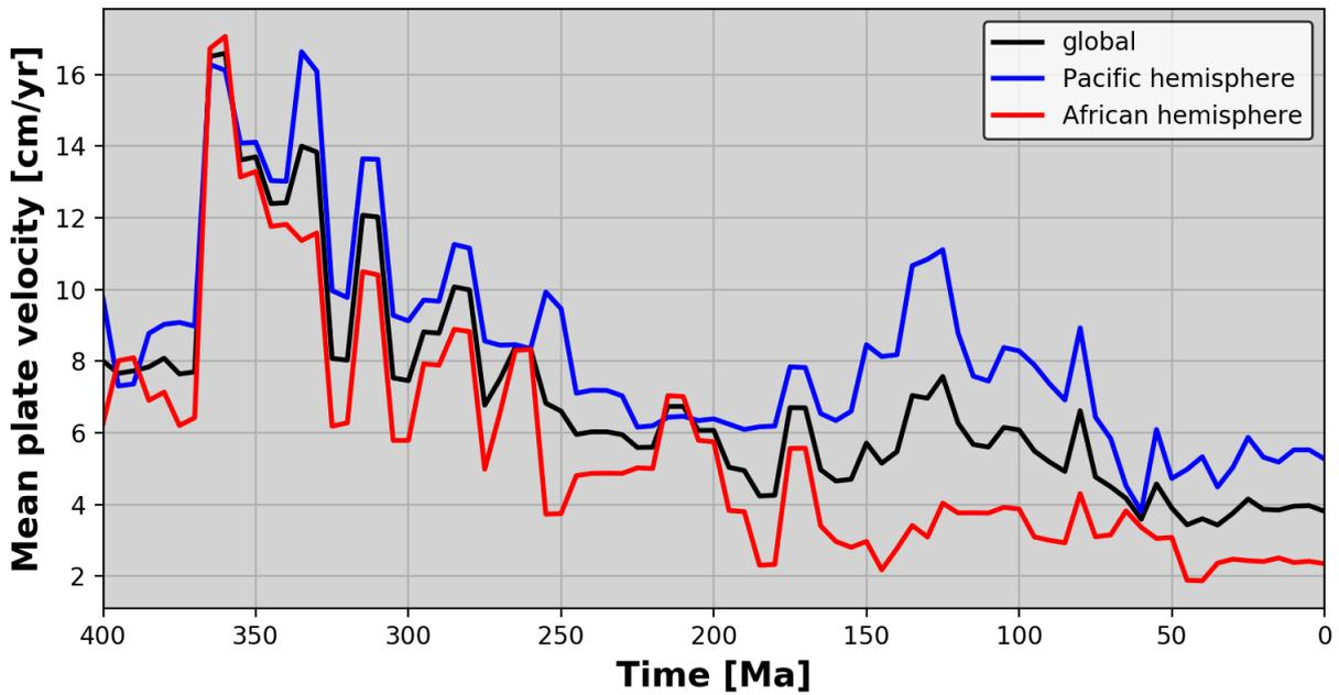
**Figure S5:** Mean plate speeds from the Pacific (blue) and African (red) hemispheres, compared to the global average (black). These are computed based on the plate tectonic reconstruction of Matthews et al. (2016), corrected after Torsvik et al. (2019).
