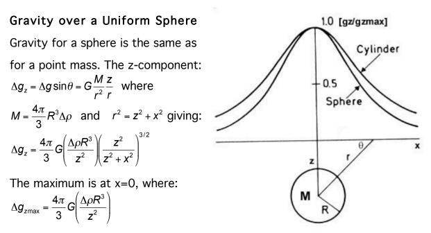
Rule of thumb: z = 0.65w where w is the width at half height of the anomaly.
